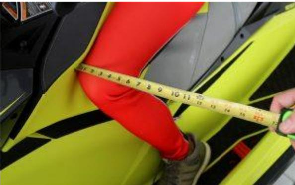
**Notebook:** This OEM seat consists entirely of soft material over the area of the rider's knee and leg. Additionally, the area of the seat is will within the 50% allowance for covering. No part of this seat assembly holds the rider in place.
