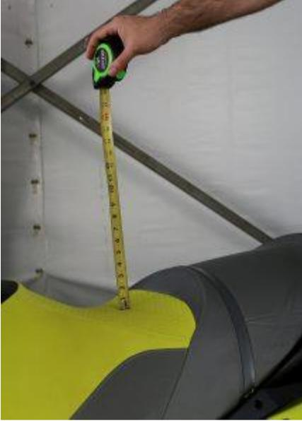
Using the lowest point of the seat a measurement is taken using the figure determined from the method above. In this case, the distance is 7.2 inches with an additional tolerance of .5 inches. The rear portion of the seat may rise 7.2 inches from the lowest point. This OEM seat is well within that allowance.
